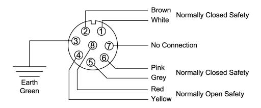
The CM-S321 is available with an IP67, 8 pole connector. Connector specification: 8-pin, Micro Single Key-way, M12 x 1  $\,$
